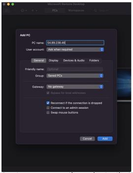
Create a new connection and enter the IP address of the newly launched EC2 Instance. For this example, the public IP address will be used as the server has been launched in a public subnet. Use the private IP address where applicable for your environment if you have a private connection into the AWS VPC of which hosts the EC2 Instance. These Private connections often take the form of a VPN connection.
